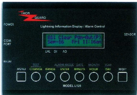
The THOR GUARD L125 utilizes our proprietary atmospheric electrostatic analysis to predict the probability of a lightning discharge within a defined area. The hyperstatic sensor connects to the L125 allowing instantaneous evaluation of the energy. The LCD indicates the storm hazard level. When the probability of a lightning discharge has exceeded your pre-selected safe level, the L125 will activate an optional LED light.
