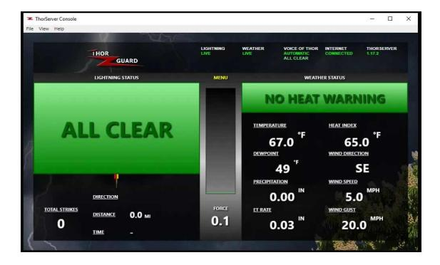
The ThorServer Software is a Windows based service software that handles and processes the TG360 Data coming down from the roof through the provided Edgerouter into the provided laptop. All the necessities are displayed on the main screen and then at first glimpse into the Menu, you'll find more settings and diagnostics for both the Weather Station and the TG360.
